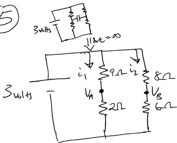
This is what the circuit looks like after an infinite amount of time has passed, i.e. no current flows through capacitor.
