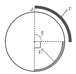
(a) (4 pts) The overlapping area between  $T_1$  and  $T_2$  is  $R\theta h$ , where  $\theta$  is the angle of overlap in radians. Given that the conductive strips cover  $\frac{1}{4}$  of the cylinder, what is the value of  $C_g$  as a function of  $\varepsilon_0$ , R, h, and d for the configuration shown below where  $\theta = \frac{\pi}{4}$ ?
