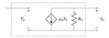
(a) (4 **pts**) For an IoTatron with an externally applied voltage of  $V_{in}$  as shown below, write an equation for  $V_{out}$  in terms of  $V_{in}$ ,  $g_m$ , and  $R_0$ .
