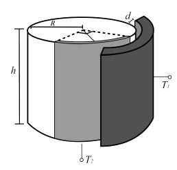
For the following problems, define  $C_g$  as the effective capacitance between  $T_1$  and  $T_2$ . You can model the capacitors here as parallel plate capacitors. You can also assume that R >> d, so that the difference in surface area between the outer and inner plates is negligible. Ignore any capacitance that is not due to direct overlap between the plates (i.e., no fringing capacitance).
