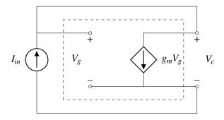
(c) (5 pts) You attach another IoTatron with  $R_o = \infty$  to the one in part (b), but this one also has a finite  $R_L$ , resulting in the circuit shown below. Solve for  $I_L$  in terms of  $g_m$ ,  $I_{in}$ , and  $R_L$ .
