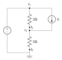
Use only KCL and Ohm's Law to set up a system of equations relating each of the labeled currents  $(I_1, I_2, I_3)$  and voltages  $(V_1, V_2)$ . Then construct a 3x5 matrix A representing this system of equations such that Ax = 0 where x is:
