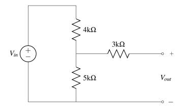
(b) (5 pts) Find  $V_{out}$  as a function of  $V_{in}$ . (Hint: Pay attention to where the positive and negative terminals of  $V_{out}$  are.)
