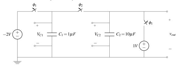
(b) (4 pts) What is the charge on each capacitor when the  $\phi_1$  switches are closed and the  $\phi_2$  switch is open? Hint: Be sure to measure the voltage across each of the capacitors in the way we have indicated on the diagram, and then pay careful attention to the signs of the charges.
