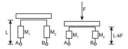
(a) (4 **pts**) Let  $R_{AB}$  be the resistance between nodes A and B. Write an expression for  $R_{AB}$  as a function of A, L,  $\rho$ , F, and k.
