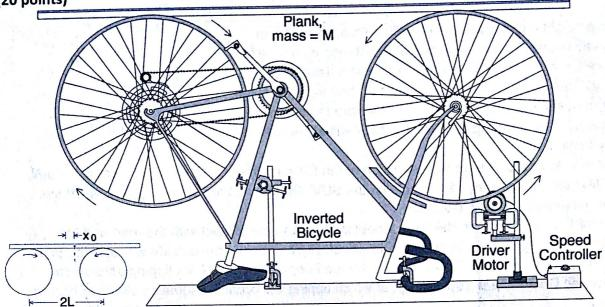
A heavy, uniform, horizontal plank of mass M rests on top of two identical bicycle wheels which are continuously turned rapidly in opposite directions, as shown. (The plank edge just fits within the curve of the rim of each wheel).
