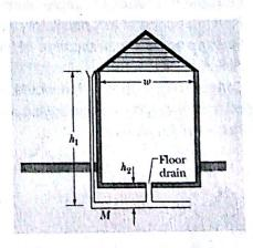
(volume of water that falls per area per time), will water from pipe M reach the height of the floor drain and threaten to go to the basement (R is small compared to  $h_1$  and  $h_2$ )?
