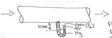
Pressure in Pipe (Pa) is to mm higher than in open arm, so Pa - Pb = - tomm Ha
