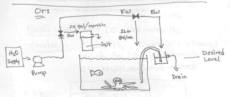
Keep Sw rate the same, add a second diverter value, keep Fw rate the Same, set "Ew" greater than evap. rate, then the "siphon" eystem shown will allow Fw to How back into tank whenever level drops below desired.
