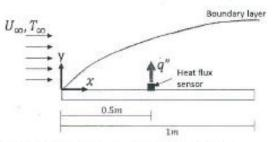
(a: 5 pts) The flow meter is specified by the manufacturer to work for  $U_{\infty}$  in the range ~10 m/s to ~100 m/s. Does this device operate in a laminar or turbulent flow regime? You must justify your answer.
