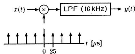
The plot below shows the Fourier transform  $Y$  of the output signal, for frequencies between 0 and 20 kHz. Write the number of the harmonic of  $x(t)$  that produced each component of  $Y$  in the box above that component. If none of 1-7 could have produced this frequency, write X.
