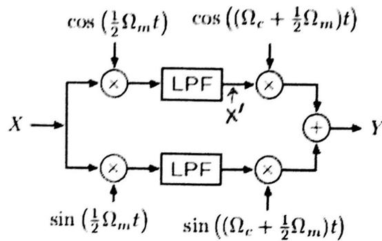
Assume that each low-pass filter is ideal, with cutoff frequency  $\frac{1}{2}\Omega_m$ . Also assume that the input signal has the following Fourier transform  $X(\Omega)$ :
