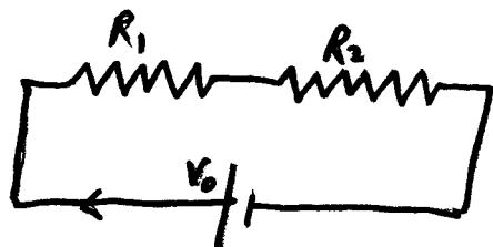
$$I = \frac{V_0}{R_1 + R_2}$$
