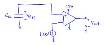
c) (12 pts) Instead of only a binary indication of the super-capacitor being almost out of usable charge, we might instead want a voltage that is linearly proportional to the remaining usable charge. Under the same constraints as part b), design a circuit that outputs 1.2V when 100% of the usable charge is left, 0V when 0% of the usable charge is left, and that drops linearly from 1.2V for any percentage in between (e.g. 0.6V for 50%, 0.3V for 25%, etc.).
