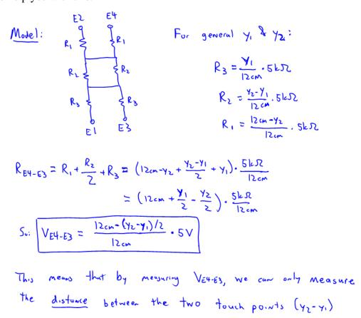
e) (**BONUS: 8 pts**) One of your colleagues claims that by measuring the appropriate voltages, not only can they extract what both  $y_1$  and  $y_2$  are in this system, they can even do so in a way that would have a set of three independent voltage equations related to  $y_1$  and  $y_2$  and hence gain some robustness to noise in the voltage measurements.
