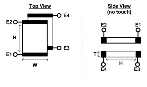
a) (4 pts) Assuming that both of the plates are made out of a material with  $\rho = 1 \ \Omega^* m$  and that the dimensions of the plates are W = 3cm, H = 12cm, and T = 0.5mm, with no touches at all, what is the resistance between terminals E1 and E2 (which would be the same as the resistance between terminals E3 and E4)?
