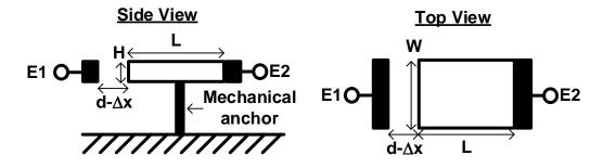
a) (3 pts) Assuming that no acceleration is applied (i.e.,  $\Delta x = 0$ ), that H=10 $\mu$ m, L=100 $\mu$ m, W = 20 $\mu$ m, d = 0.5 $\mu$ m, and that the proof mass is made out of nickel (i.e., a conductive metal), what is the capacitance between E1 and E2?
