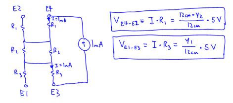
f) (**BONUS: 8 pts**) Using the equations you derived in part e), show the procedure you would use to estimate  $y_1$  and  $y_2$ . Note that your final result should be in the form of a matrix-vector equation that predicts  $y_1$  and  $y_2$  as a function of the measured voltages. (Note that you can plug in numbers for all of the dimensions/material constants such as H, L, etc.)
