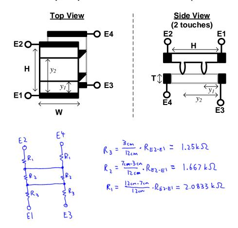
c) (6 pts) Using the same assumptions as part b), if you drove terminals E3 and E4 with a 1mA current source (as shown below) but left terminals E1 and E2 open-circuited, what is the voltage you would measure across E4-E3 (i.e.,  $V_{E4-E3}$ )?
