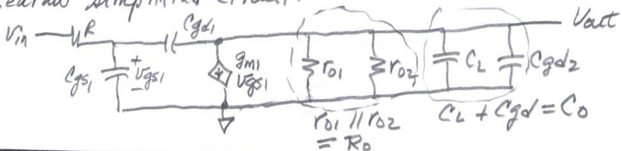
$$\omega_p = \left[ R C_{gs1} + R_o C_o + (R_o + R + g_m1 R_o R) C_{gd1} \right]^{-1}$$
