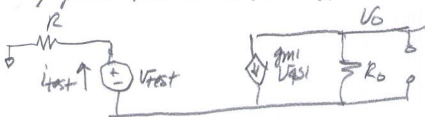
$$\frac{V_{test}}{i_{test}} = R \therefore \Sigma_4 = R C_x = R (C_{gs1} + C_{gd1} (1 + g_{m1} R_o)) \quad \leftarrow \Sigma_1$$
