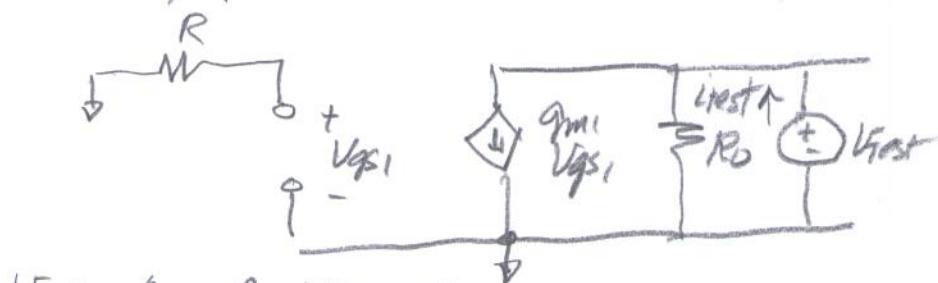
$$V_{gs1} = 0 \therefore g_{m1} V_{gs1} = 0$$
