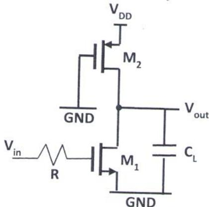
First, draw the complete small-signal model for M<sub>1</sub> and M<sub>2</sub>
