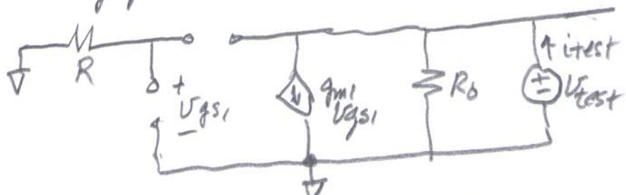
$$V_{GS1} = 0 \quad \therefore g_m, V_{GS1} = 0 \quad \therefore \frac{V_{test}}{i_{test}} = R_o \quad \therefore Z_2 = R_o C_o$$
