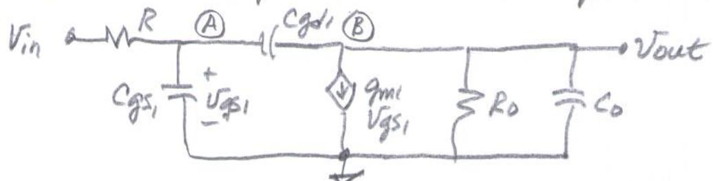
Note:  $C_{gd1}$  is connected between  $\textcircled{A}$  and  $\textcircled{B}$  so we need to find the voltage gain from  $\textcircled{A}$  to  $\textcircled{B}$ .
