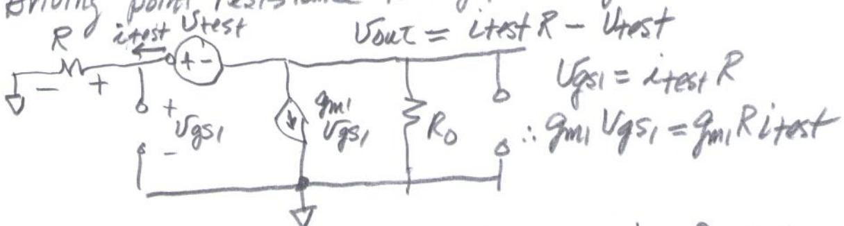
• KCL at  $V_{out}$ :  $i_{test} + g_m R i_{test} + g_o i_{test} R - g_o V_{test} = 0$
