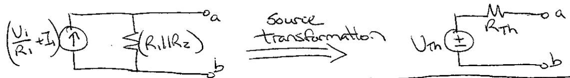
$U_{Th} = \left(\frac{V_1}{R_1} + I_1\right)(R_1 || R_2) \Rightarrow U_{Th} = \left(\frac{V_1}{R_1} + I_1\right)\left(\frac{R_1 R_2}{R_1 + R_2}\right)$
