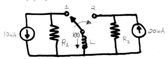
The switch in the circuit below was moved from position 1 to position 2 at t = 0. Prior to t = 0, it was at position 1. L = 80 mH.  $R_1$  = 20  $\Omega$ ,  $R_2$  = 40  $\Omega$
