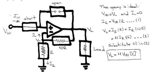
Fraw in components in all boxes below so that the voltage across **the load** is exactly **-10**Im [V]. You can place the load in any box. In addition to the ONE load, you may use TWO resistors and ONE of everything else. (7.5 points)
