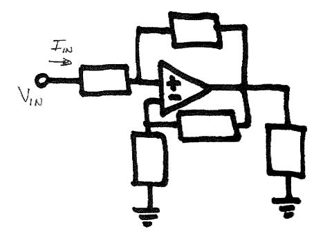
c) Draw in components in all boxes below so that the voltage across **the load** is exactly  $V_L = -10I_{IN}$  [V]. You can place the load in any box. In addition to the ONE load, you may use TWO resistors and ONE of everything else. (7.5 points)
