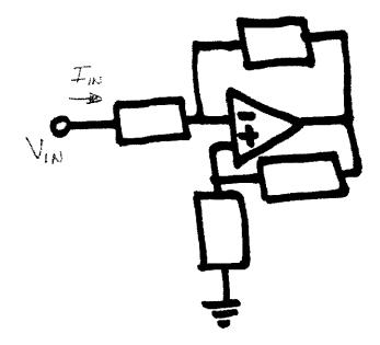
b) Draw in components in all boxes below so that the voltage across **the load** is exactly  $V_L = 11V_{IN}$  [V]. You can place the load in any box. In addition to the ONE load, you may use TWO resistors and ONE of everything else. (7.5 points)
