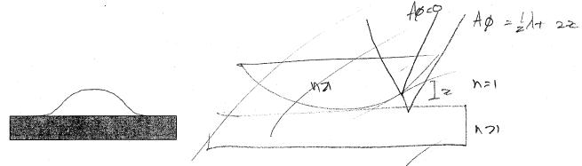
4) An oil drop (n = 1.2) floats on a water (n = 1.33) surface and is observed from above by reflected light.
