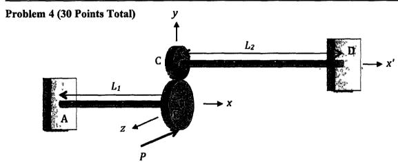
A mechanism (not shown) below gear B exerts a force P on that gear. Force P is parallel to the z axis. Shaft AB is fixed at A and has length  $L_I$ ; shaft CD is fixed at D and has length  $L_2$ . Both shafts have the same polar moment of inertia J and are made of the same material with shear modulus G. Gear B has a radius of  $r_B$  and gear C has a radius of  $r_C$ .
