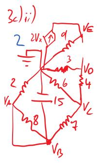
$V_x = V_c - V_B$ = 12-15  $V_{B} = 15V \Lambda$  $\frac{V_{\text{E}}}{a} - 2V_{\text{x}} = 0$ VA = VB = 15V 1  $V_{E} = -2(V_{c} - 15) = 0$  $\frac{V_{c}-15}{2} + \frac{V_{c}}{4} + \frac{V_{c}-V_{0}}{4} = 0$ VE-18Vc=-270 47VC-21VD=15×12=180IN <u>\_</u><u>\_</u>  $\frac{V_0}{3} + \frac{V_0 - V_c}{4} = 0$ -3V2+7V2=0D1
