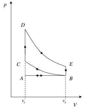
4. The thermo dynamical cycle to the left is the cycle likely used by your car. Find the total work, *W*, done in a complete cycle (expressed in terms of the pressure at *B*, *C*, *D*, and *E*, and the volume at *A* and *B*), and the efficiency, *e*, of the cycle (expressed in terms of the temperature at *D* and *E*). The gas used has a given value of *γ*.
