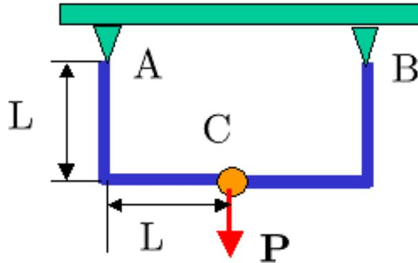
Figure 2: A three-hinge arch truss system
