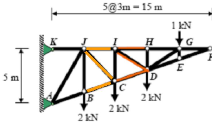
Figure 1: A truss structure under multiple loads
