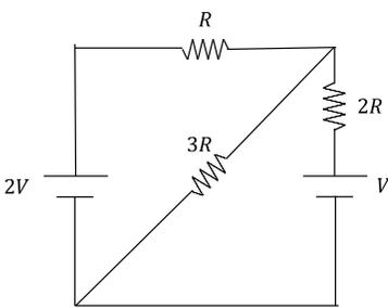
5. For the circuit on the left, find the current,  $I$ , through the resistor,  $3R$ , in terms of  $V$  and  $R$ .
