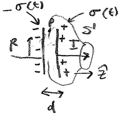
$$\textcircled{b} \quad \vec{J}_d = \epsilon_0 \frac{\partial \vec{E}}{\partial t} = -\frac{\partial \vec{B}(t)}{\partial t} \hat{z} \quad \left( \frac{\partial \vec{B}}{\partial t} \angle 0; \vec{J}_d \text{ points to right} \right)$$
