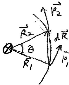
a)  $\vec{F}_q = q \vec{v} \times \vec{B} = -q v B_{\text{orb}} \hat{r}$
