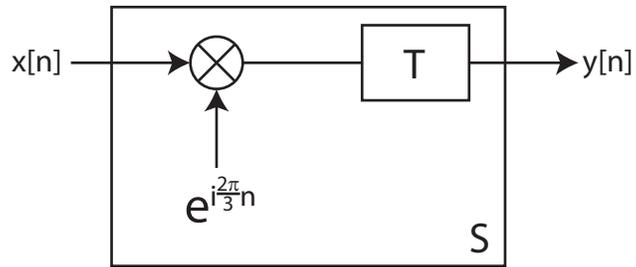
Shown above is a discrete time system  $S$  with input  $x[n]$  and output  $y[n]$ . The LTI system  $T$  inside  $S$  is causal and has impulse response  $h[n]$ .
