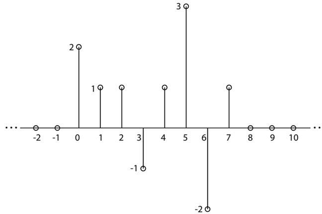
Given a discrete time sequence  $x[n]$  shown above (note  $x[n]$  is non-zero only for  $0 \leq n \leq 7$ ):
