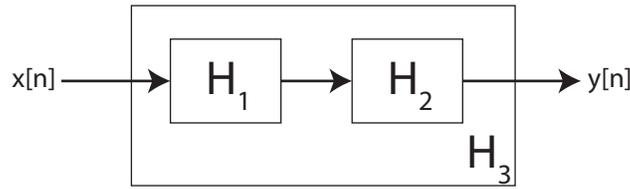
System  $H_1$  has the LCCDE  $y[n] = \alpha_1 y[n-3] + x[n]$ . System  $H_2$  has the LCCDE  $y[n] = \alpha_2 y[n-6] + x[n]$ .
