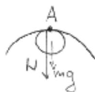
$N + mg = m \frac{v_A^2}{R_A}$        $R_A$  max for  $N \rightarrow 0$
