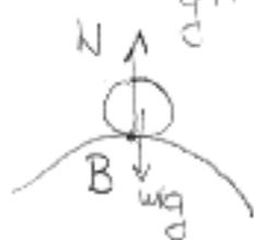
$m \frac{v_B^2}{R_B} = mg - N$        $R_B$  min for  $N \rightarrow 0$
