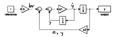
Assume the initial conditions of both the integrator blocks  $(\frac{1}{s})$  are zero. Write the SLODE model (linking y to r) for this diagram.
