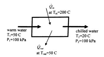
energy, and the water can be approximated as incompressible with specific heat 4.2 kJ/kg K. Neither  $\dot{Q}_{in}$  or  $\dot{Q}_{out}$  is specified.
