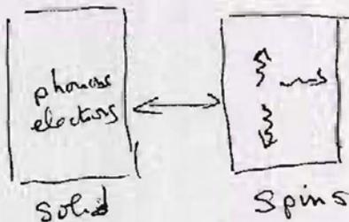
When we decrease adiabatically the magnetic field  $B$ , the entropy of the spins tends to increase - Therefore the entropy of the solid has to decrease. The temperature of the solid and spins decrease!
