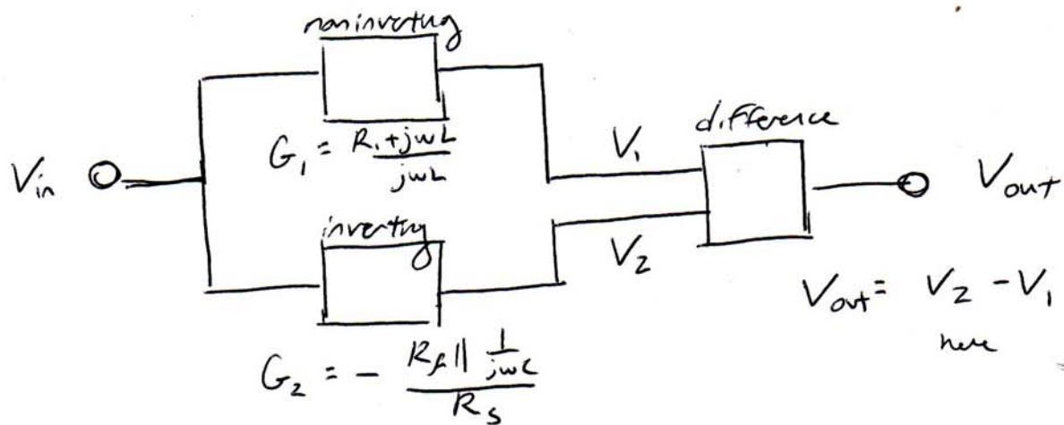
$$\therefore V_{out} = V_2 - V_i = \left( -\frac{R_f}{R_s} \frac{1}{(1+j\omega R_f C_f)} - \frac{R_i + j\omega L}{j\omega L} \right) V_{in}$$
