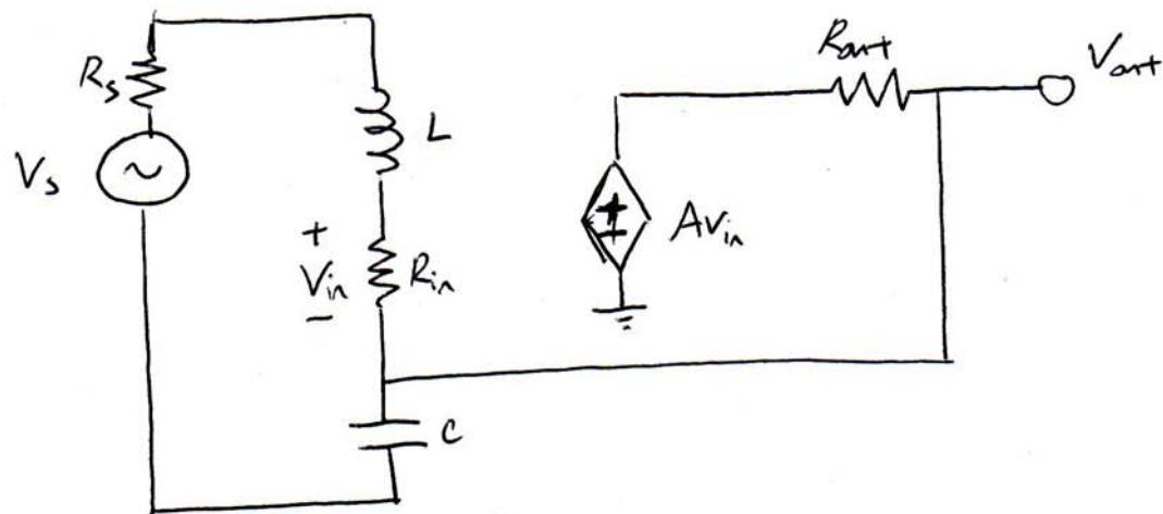
$V_{out}$  follows phase of  $A V_{in}$  since  $R_{out}$  is purely real.
