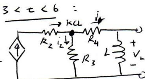
$$\begin{aligned} \beta V_c &= i_L + i_2 = i_L + \frac{(i_L R_3 + L \frac{di_L}{dt})}{R_3} \\ &= i_L \left( \frac{R_3 + R_4}{R_3} \right) + \frac{L}{R_3} \frac{di_L}{dt} \end{aligned}$$
