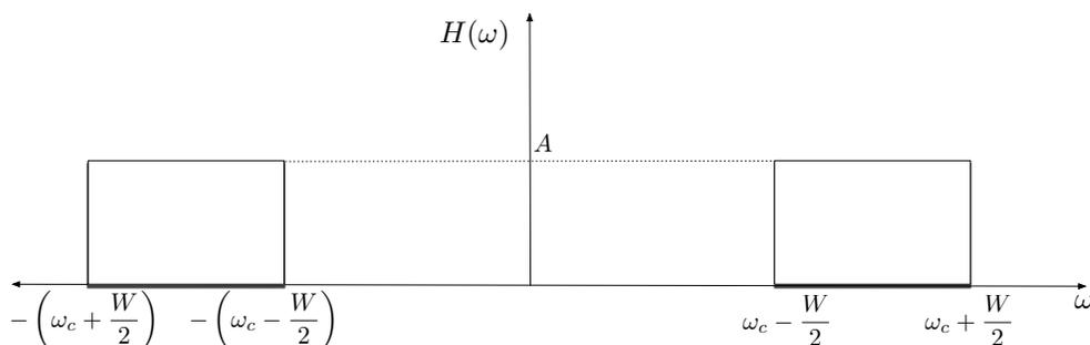
Figure 4: Frequency Response Magnitude. Phase is zero throughout.
