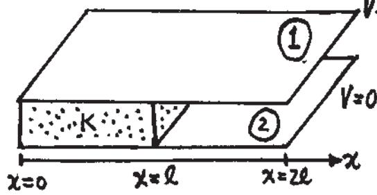
$V = V_0$  of  $V_0$  volts between them. Half of the volume between the plates is then filled with a dielectric of dielectric constant  $K$  (shown dotted in the figure).
