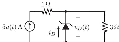
Evidently, the Zener diode is now reverse-biased. On the plot below, draw in the load line immediately after the current source turns on, i.e.,  $t = 0_+$ . Be sure to label slopes and intercepts; your plot need not be to scale.
