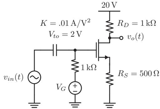
(a) (10 points) Recall that the transconductance of the transistor is given by
