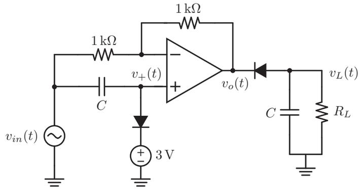
(b) (5 points) Find an expression for  $v_o(t)$  in terms of  $v_+(t)$  and  $v_{in}(t)$ .
