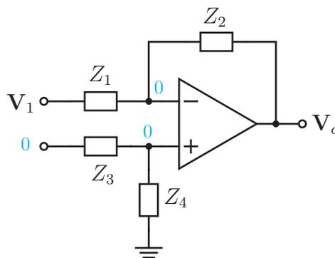
This is simply an inverting amplifier. Therefore, the contribution from  $\mathbf{V}_1$  to  $\mathbf{V}_o$  is determined to be:
