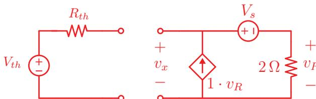
Now we are able to use nodal analysis to find  $V_{th}$  and  $R_{th}$ . Using a supernode, we get the following two equations:
