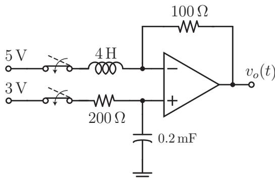
(a) (8 points) Find  $v_+(t)$  at the noninverting input for  $t > 0$ .
