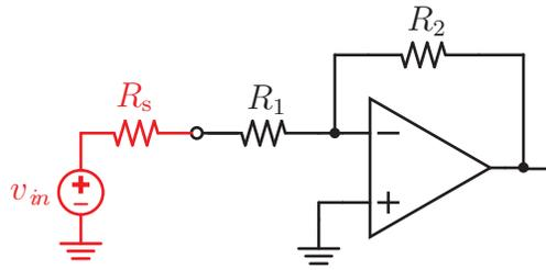
We can model the source as shown above. Solving the circuit with SPC and KCL, the gain of the first stage (inverting op-amp configuration) becomes  $G_{inv} = -\frac{R_2}{R_1 + R_s} = -\frac{10 \text{ k}\Omega}{100 \Omega + 10 \text{ k}\Omega} \approx -1$ . Therefore, the total gain drops significantly.
