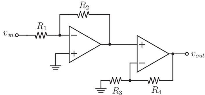
This is cascade of inverting op-amp and non-inverting op-amp. The gain is
