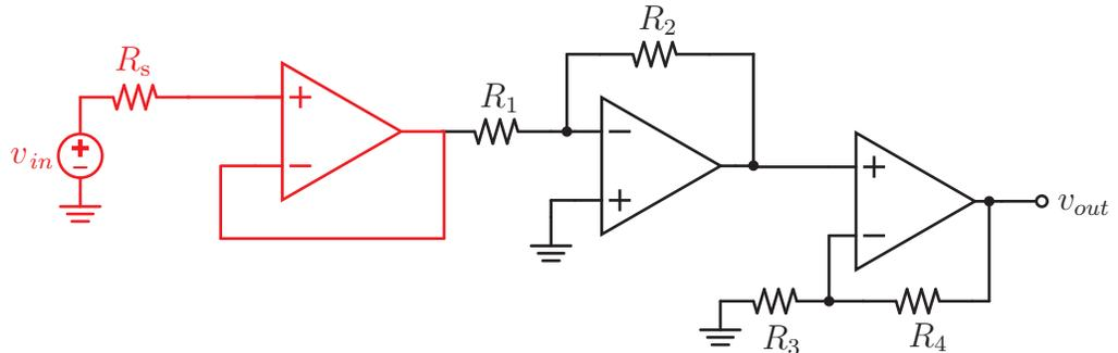
To solve the problem of impedance matching, we can insert a voltage follower as shown above (infinite input resistance with a gain of 1, ideally) at the beginning of the circuit. Now the gain is not affected by the source resistance and stays at -10100. The tradeoff of adding another stage, of course, is that the circuit now consumes more power and takes up more space.
