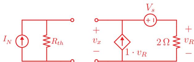
Here we will do the Norton equivalent circuit. The two equations from the supernode around  $V_s$  is as follows:
