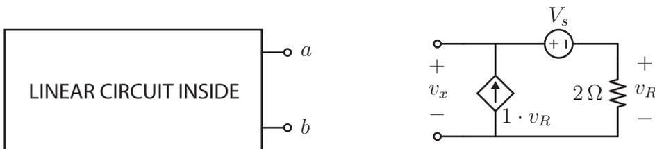
Instead of having a multimeter like normal people, John has the above whack measuring device (shown on the right). The device can be attached across two terminals of any circuit. The value of  $V_s$  can be twiddled with, and the device will then report the voltage  $v_x$ .
