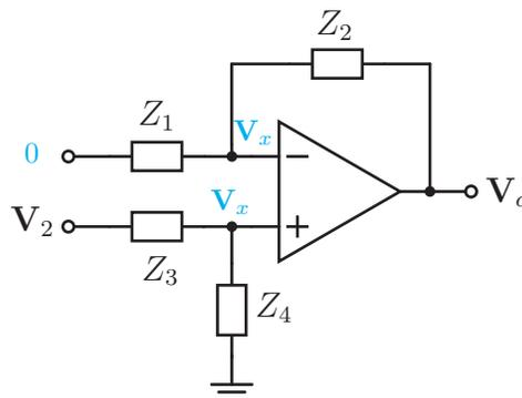
We recognize that this is a non-inverting amplifier and therefore the gain is determined to be:
