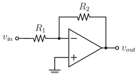
This is an inverting op-amp configuration. The gain is simply  $G = -\frac{R_2}{R_1}$ .
