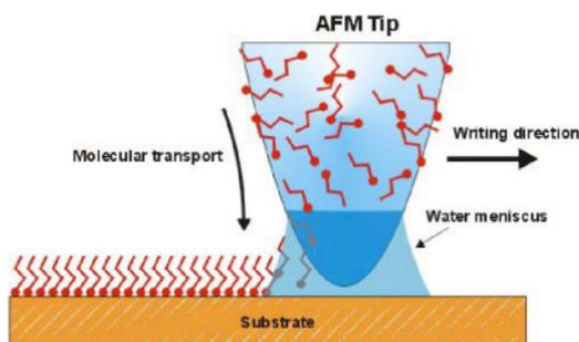
DPL is a direct-write scanning probe-based lithography. An AFM tip is used to deliver chemical reagents (peptides) to nanoscopic regions of a target substrate where they can self assemble. Desired chemistry is carried out exactly where it is needed.
