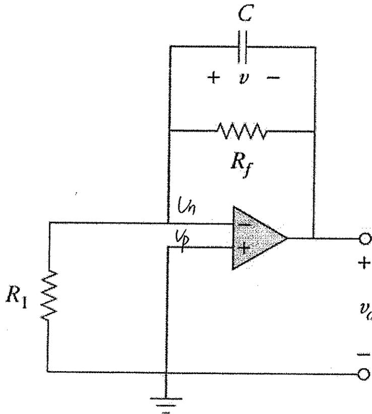
$$V_o = -V(0) e^{-\frac{t}{R_f C}} \quad (V) \quad t > 0$$
