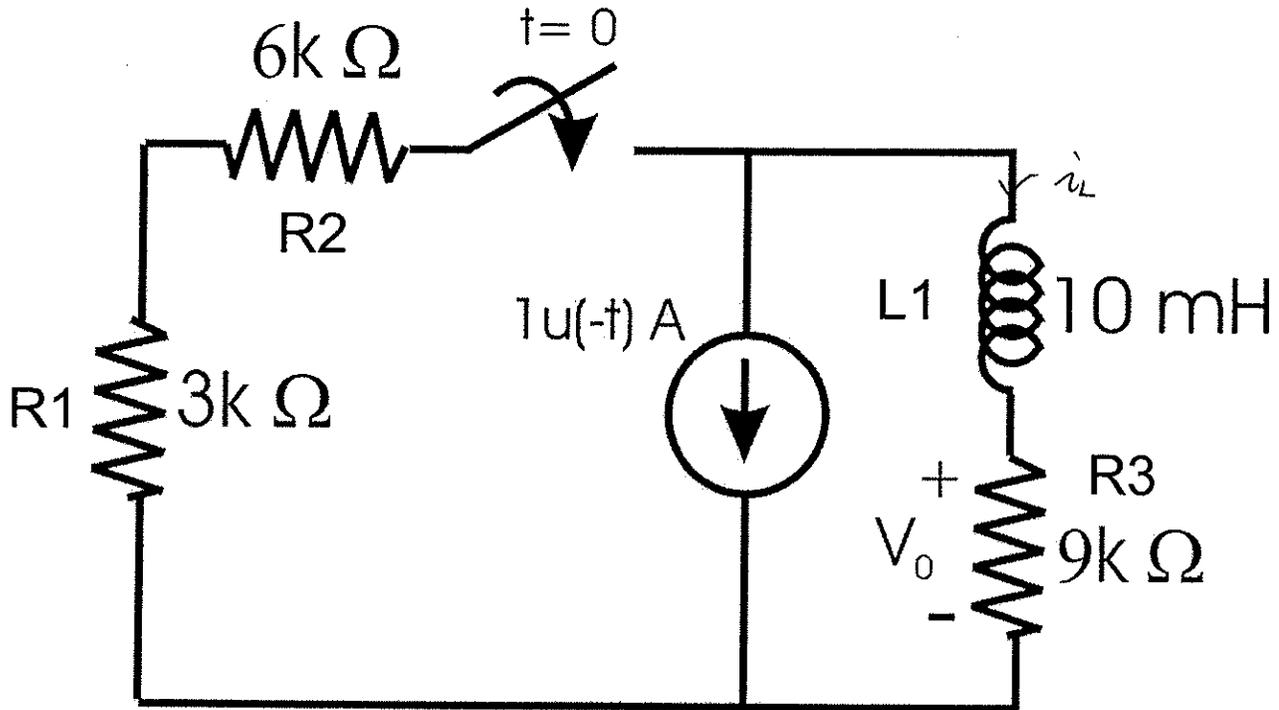
a) What is the value of  $V_0$  at  $t = 0^+$ ? Write It in the BOX BELOW. (5 points)
