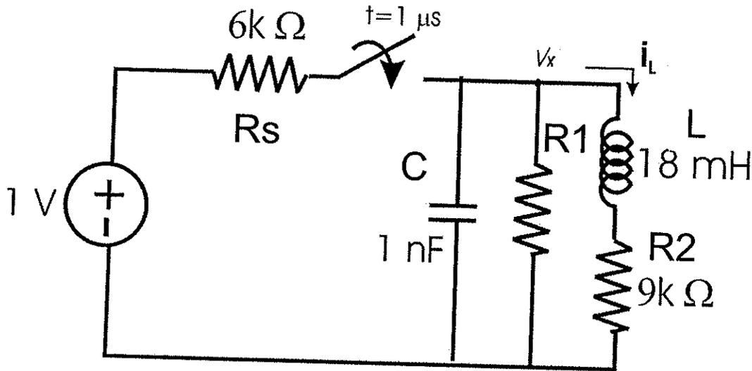
a) Find the second order **differential equation** for the variable  $i_L$  that describes the circuit behavior for  $t > 1 \mu s$ . Write into the box below. (15 points)
