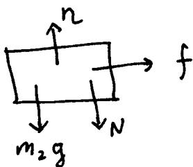
here  $f$  is static friction force due to surface between blocks.
