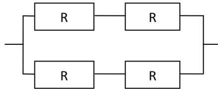
The effective resistance can be found by summing the resistors in the above diagram, which gives:
