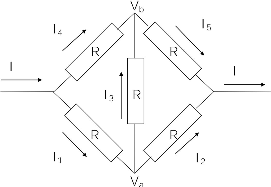
But after the reflection, the assembly of these 5 resistors looks exactly the same as before. Hence they are the same circuit.
