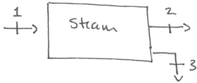
$$\left. \begin{array}{l} P_1 = 2.0 \text{ MPa} \\ T_1 = 250^\circ\text{C} \\ \dot{m}_1 = 0.60 \text{ kg/s} \end{array} \right\} \begin{array}{l} h_1 = 2903.3 \text{ kJ/kg} \\ s_1 = 6.5475 \text{ kJ/kg-K} \end{array} \quad P_3 = 0.10 \text{ MPa}$$
