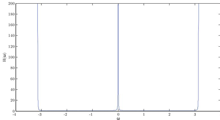
Figure 2: The system's frequency response for  $\alpha = 0.99$  in 1(c). The important labels are  $\omega = 0, \pi, -\pi$ .
