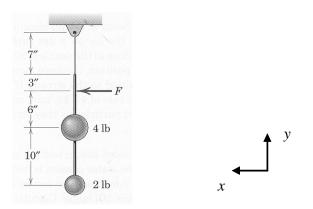
Let G be the center of mass of the system. Upon application of the horizontal force F, G will move with an acceleration  $a_G$  in the direction of F. From the generalized equation of motion,
