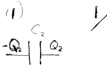
2  $C_2 = \frac{Q_2}{V_2} \Rightarrow V_2 = Q_2 / C_2$  2/
