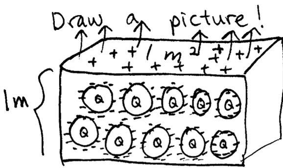
What's going on: Charges inside cavities attract negative charges from the conductor. Since the conductor is originally neutral, then an equal amount of positive charge must accumulate on the outside surface of the slab.
