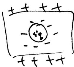
→ needed to mention/draw negative charge on inner surface of cavity balanced by positive charge on outside of conductor.
