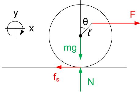
**Linear Dynamics.** We draw the free body diagram as shown, making careful note of the fact that we have defined *clockwise* as positive rotation. We write down the linear dynamics equation,
