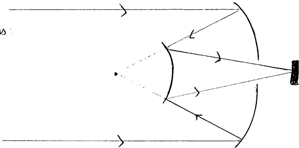
b) We are asked to calculate  $d_{i,s}$ , the image distance of the secondary mirror, since that is where a star will be in focus.
