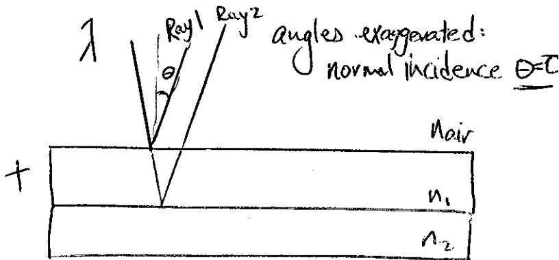
Suppose  $n_2 > n_1 > n_{\text{air}}$ . Then we see an interference maximum for  $\lambda_1 = \lambda$ , which means that compared to Ray 1, Ray 2 travels a longer path by a ~~fixed~~ distance  $PD = m\lambda$  for  $m=1,2,\dots$
