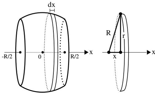
We cannot use any formula directly (such as  $R = \rho l/A$ ) to calculate the resistance of this geometry directly since the cross sectional area changes as the current moves inside the conductor. But we can break the truncated sphere into tiny discs, each with resistance  $dR$ , assume that the current flows uniformly through these discs, and calculate the total resistance  $R$  integrating.
