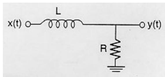
a) Derive the differential equation relating  $x(t)$  and  $y(t)$ .
