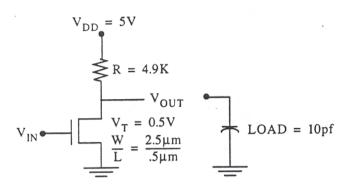
Note: For this transistor  $C_{ox} = 10 \text{fF}/\mu \text{m}^2 = 1 \mu \text{F/cm}^2$   $\mu = 1000 \frac{\text{cm}^2}{\text{V sec}}$  for electrons
