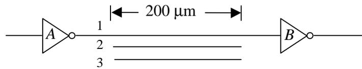
Inverters A and B:  $R_n = R_p = 100 \Omega$   $V_{DD} = 2.5 \text{ V}$
