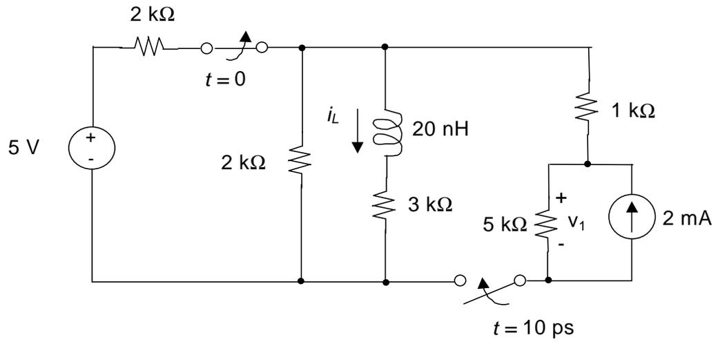
(a) [4 pts.] What is the numerical value of the inductor current  $i_L(0)$  when  $t = 0$ .
