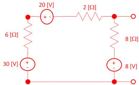
Step 2: Combine the sources and resistors on the left and top side of the circuit
