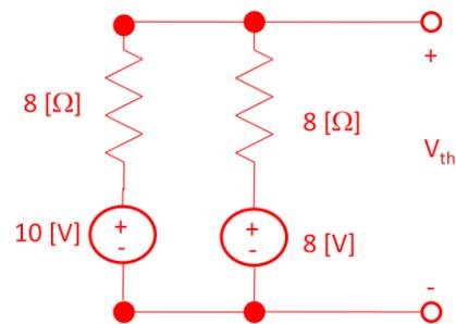
Step 3: Now utilize the voltage divider relation to solve for  $V_{th}$
