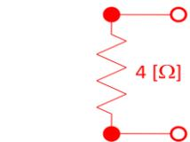
$$\text{Parallel: } R_{eq} = \frac{R_1 \cdot R_2}{R_1 + R_2} \quad : \quad R_{eq} = \frac{8\Omega \cdot 8\Omega}{8\Omega + 8\Omega} = 4\Omega$$
