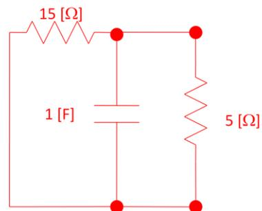
$$R_{eq} = \frac{15[\Omega] \cdot 5[\Omega]}{15[\Omega] + 5[\Omega]} = \frac{75}{20} [\Omega]$$
