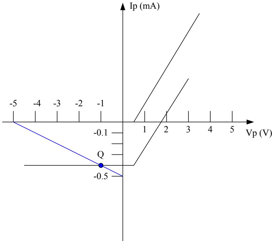
(b) Given the  $v_{GS}-i_D$  characteristics of the MOSFET which is shown in the  $v_{GS}-i_D$  plot below, please draw the load line on this plot, label the operating point Q of the MOSFET and give  $v_{GSQ}$  and  $i_{DQ}$  values of the operating point. [10 pts]
