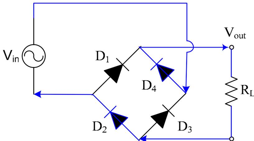
$D_2$  and  $D_4$  are on while  $D_1$  and  $D_3$  are off. So  $V_{out}$  on the load resistor is  $V_{in}$  positive half cycle.
