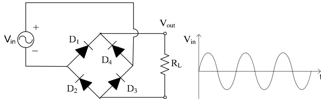
(a) Please draw the output voltage on the load resistor and give explanations. (The input is given as a reference.) [8 pts]
