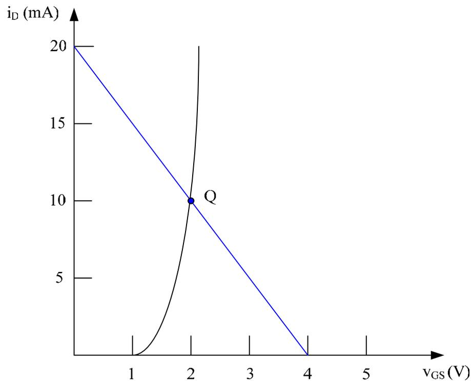
(c) Given the  $v_{DS}$ - $i_D$  characteristics of the MOSFET which is shown in the  $v_{DS}$ - $i_D$  plot below, please draw the load line on this plot, label the operating point Q of the MOSFET and give  $v_{DSQ}$  value of the operating point. [10 pts]
