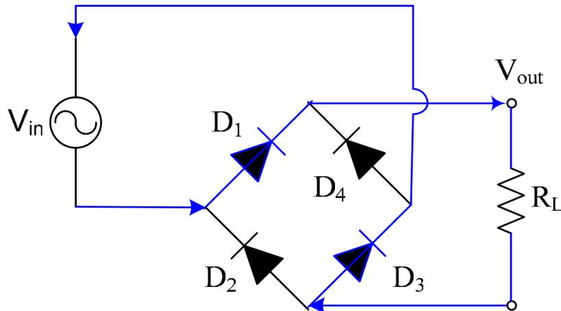
$D_1$  and  $D_3$  are on while  $D_2$  and  $D_4$  are off. However, the current goes through the resistor in the same direction. So  $V_{out}$  on the load resistor for the negative half cycle is the same as it was for the positive half cycle.
