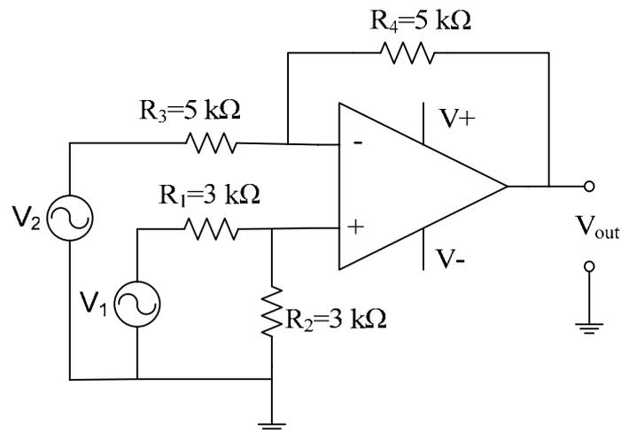
(a) Express  $V_{out}$  in terms of  $V_1$  and  $V_2$ . [5 pts]
