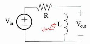
Using complex impedances, derive the transfer function  $H(\omega)=V_{out}/V_{in}$  as a function of R and L (6 pts)
