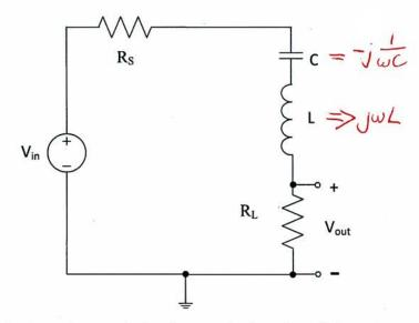
(a) Using complex impedances, derive the transfer function  $H(\omega)=V_{out}/V_{in}$  as a function of  $R_s$ , C, L and  $R_L$ . (12 pts)
