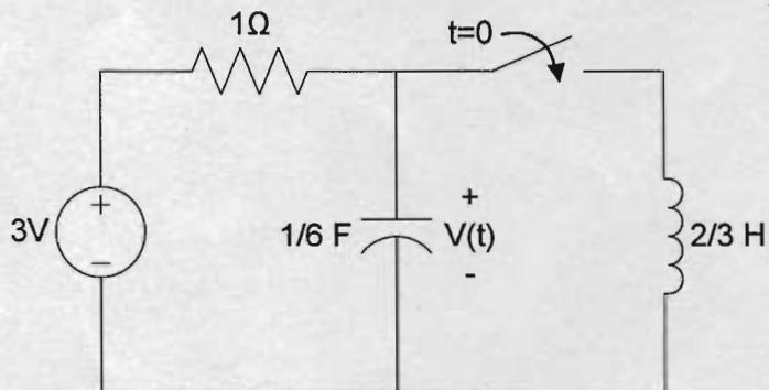
The switch is closed at  $t=0$ . The goal is to find the voltage across the capacitor,  $V(t)$ .
