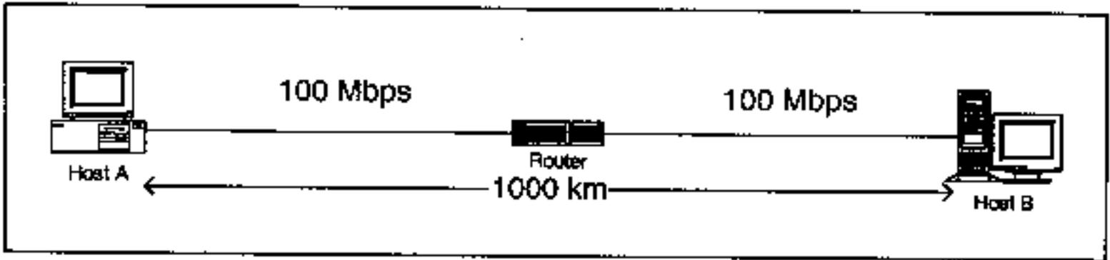
Host A sends 1500-byte packets to host B using TCP. Host B sends back ACKs. We assume that the hosts are very fast and have huge memories. What is the minimum size of the memory that the router must make available to the packets from host A to be able to sustain the maximum throughput from A to B? Explain your answer carefully.
