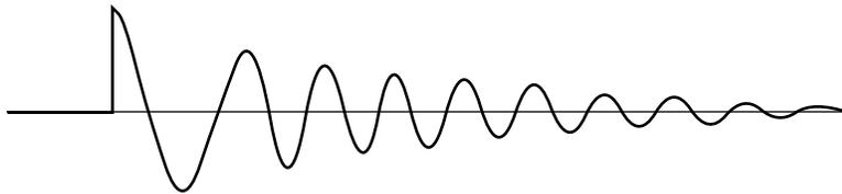
Figure 1 Impulse response  $c(t)$  = the sum of a decaying exponential and a decaying cosine wave.
