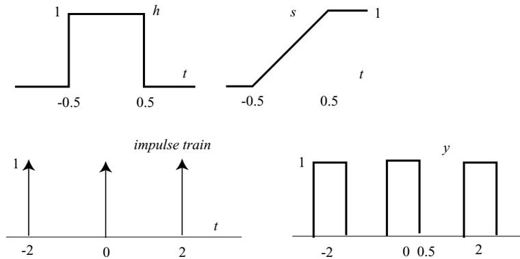
Figure 5: Impulse response, step response, impulsetrain and response for Problem 8
