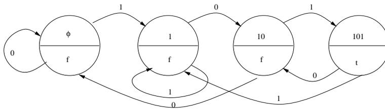
Figure 3: Required state transition diagram.
